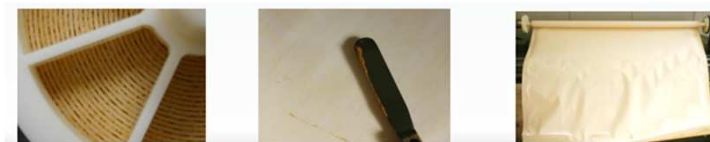
Figure 2: Autopsied NF membrane, the fouling layer is visible in the middle. Due to the presence of the fouling the flux declined from reference 42 to 12 l/m 2 .h. Cleaning tests revealed irreversibility of the fouling with a maximum improvement to 19 l/m 2 .h. Analysis of the fouling showed biofouling, mostly consisting of hydrocarbons (70%) from which 31% aromatic hydrocarbons.
