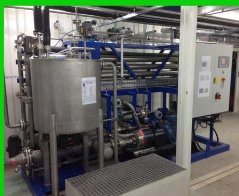
First industrial unit , based on tubular Nano Filtration + MBR + Activated Carbon. 16 ton/day, designed as containerized system 'plug in and start-up'. Build in Europe by SME's. First unit running in P&G China since Feb 2015; more than 3000 ton of high concentrated wash water treated.
